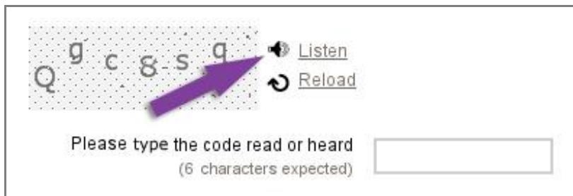
Figure 40: in this CAPTCHA, the link “Listen” provides the user with a sound version of the CAPTCHA.
